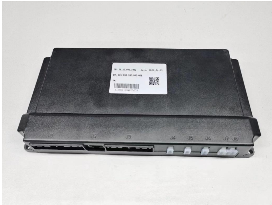
Overview of BCU box
